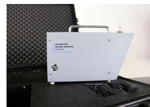
Salt particulate Generator
