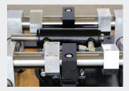
One twin rod cylinder per direction
