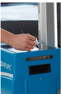
Touch screen | Ports : USB, series, RJ45, and wireless
