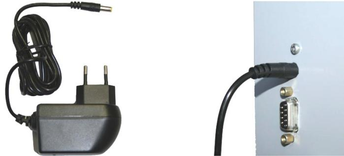
Battery charge is shown through continuous lighting of the battery light. When the light is off, the batteries are charged and then you can disconnect the charger.
