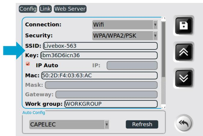
For networks with DHCP, keep the "IP AUTO" configuration, otherwise switch to static IP by unchecking "IP AUTO" and enter an IP address
